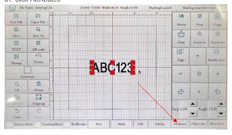
9. Adjust marking speed: 100-3000mm/s, laser power: 10-100%. Other parameters do not adjust, apply, exit
