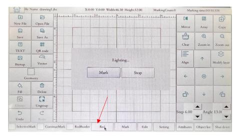
11. The laser head will display the marking position in the red frame, which means where to hit, and the size of the frame will be as large as the text
