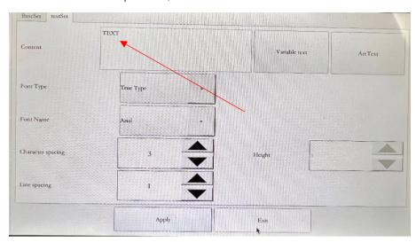
4. Enter the marking content, the position pointed by the arrow is the cycle key (lowercase, uppercase, Chinese, traditional), and confirm after input.
